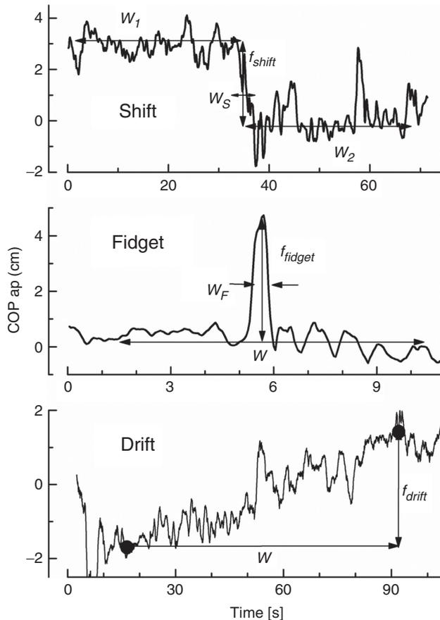
Figure 10.6 An example of shifting, fidgeting, and drifting patterns during prolonged unconstrained standing, with the corresponding parameters used for identification.
