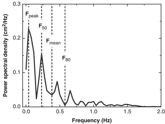
Figure 10.3 Example of the power spectral density estimation of center of pressure (COP) displacement during quiet standing. The peak ( $F_{\text{peak}}$ ), mean ( $F_{\text{mean}}$ ), and median ( $F_{50}$ ) frequencies and the frequency band that contains up to 80% of the power spectrum ( $F_{80}$ ) are also shown.
