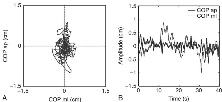
Figure 10.2 Examples of *statokinesigram* (A) and *stabilogram* (B) of center of pressure (COP) displacement during standing as still as possible on a force plate.
